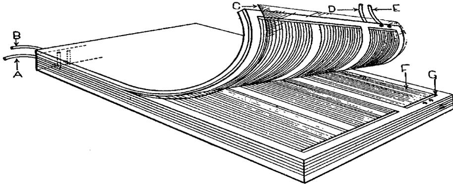
Figure 7: Flat plate kidney using Kiil membranes, c. 1965.
